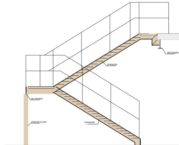
Elevation - Single Flight Staircase
