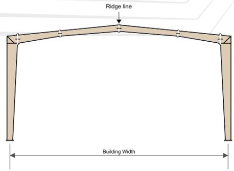
**Tapered Column Clear Span (TCCS)**
