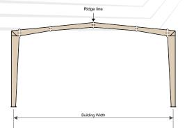
**Tapered Column Clear Span (TCCS)**
